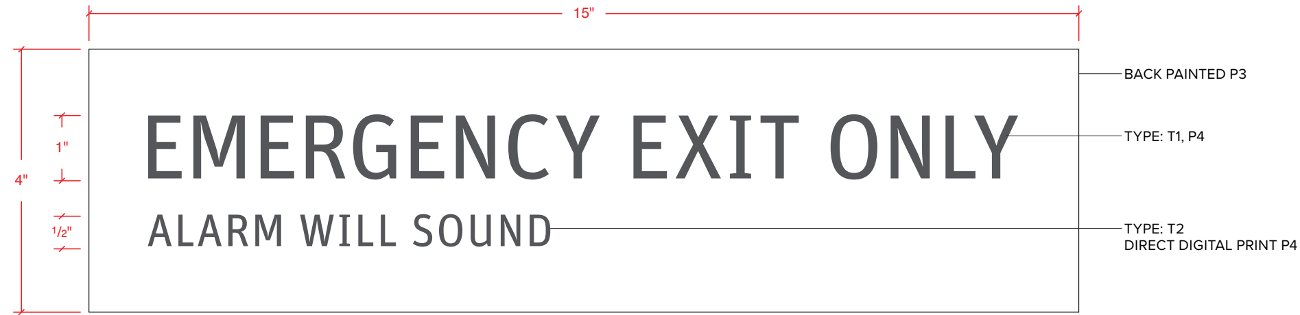
1 Detail - 12 Emergency Exit ID Scale: 1/2 Full Size
