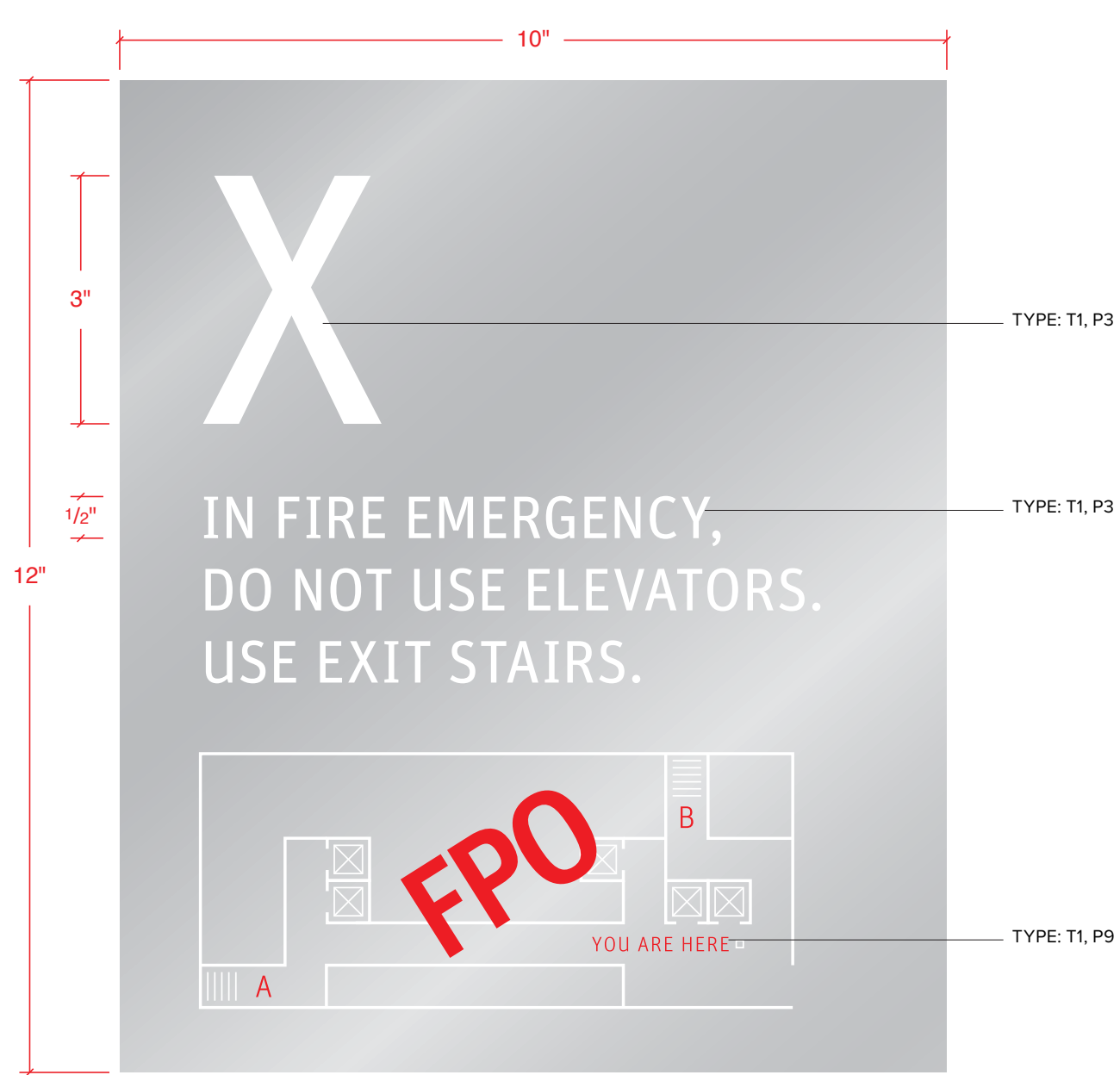
1 Detail - 20 Elevator Egress Scale: 1/2 Full Size QTY: 4
