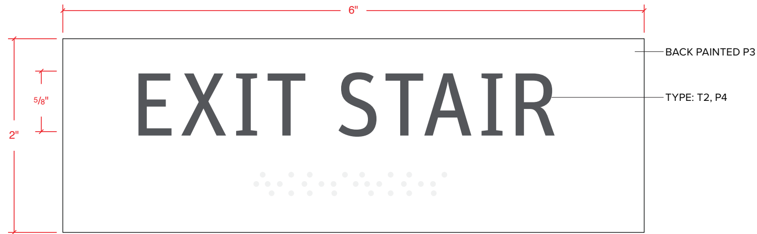
1 Detail - 11 Exit Stair ID Scale: Full Size
